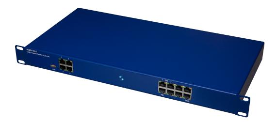
SpliceCom's 5500 Network Service Gateway provides full remote site survivability for up to 250 users in the event of primary IP trunk failure to centralised S8000 and 5100 based Call Server systems. Also provides local call breakout across ISDN BRI, PRI and/or SIP trunks and connectivity of legacy DPNSS systems and services, alongside support for analogue telephones and fax machines.
